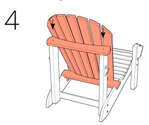
Slide the back into place and fasten it to the the back legs, using 2 short bolts.
