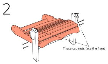
Attach the front legs to the seat. Ensure the legs are facing the direction shown. Fasten with 4 long bolts.
