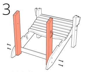
Attach the back legs to the seat, using 4 short bolts.
