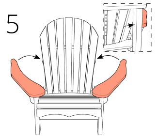
Match the key-holes on the arms onto the front legs. Make sure the arms are level on the top of the legs before pivoting them 30° into place. Bolt the arms onto the back legs with 2 long bolts.
