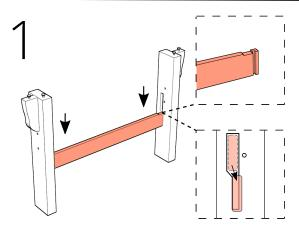
Insert the front leg support between the front legs, sliding it all the way down.
