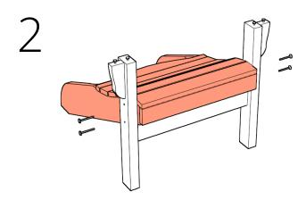
Attach the seat to the front legs using 4 long bolts.
