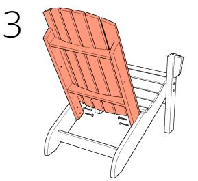
Slide the back into place and secure it to the seat using 4 short bolts.
