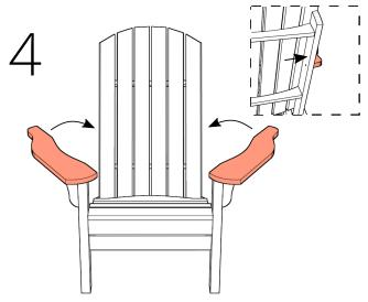
Match the key-holes on the arms onto the front legs. Make sure the arms are level on top of the legs before pivoting them 30° into place. Bolt the arms onto the back legs with 2 short bolts.
