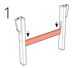
Insert the front leg support between the front legs. Lightly use a mallet if necessary.
